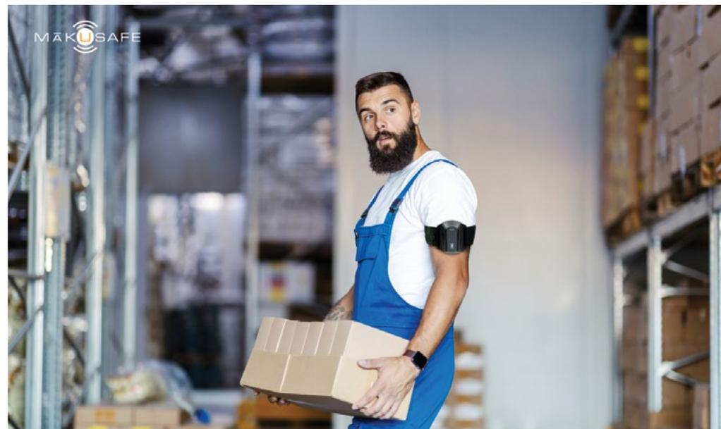
MakuSafe’s sensor-packed wearable not only detects slips and falls but repetitive motions and worker physicality. (photo courtesy MakuSafe)
