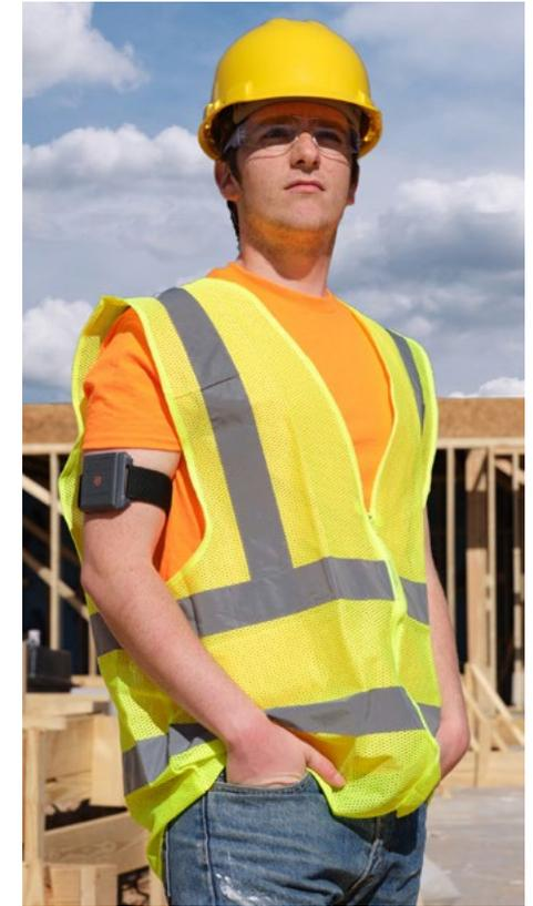
rugged conditions, it provides a bevy of functionality including worker physiological monitoring, real-time location status, automated work/rest cycles and more.
